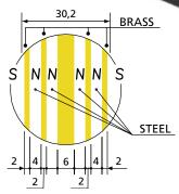
The fine pole pitch grants extremely tight magnetic closing (approximately 5mm) that allow the maximum clamping force even on small thickness pieces.
